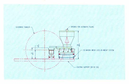
This system consists of two components: Crescent MagnaWeigh Loss-In-Weight Feeder and Crescent Electromagnetic Vibratory Spreader Feeder. These components are described in the following:
